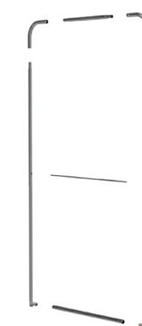
2 Add the central reinforcement tube and connect all the tubes according to the numbered system
