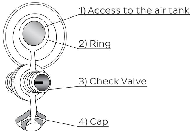
**1)** Inflate the furniture at 60% with the **access to the air tank**. Then reajust the cover easily.
