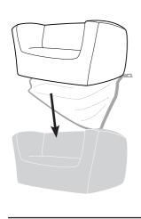
**4)** Put the cover string in the eyelets of the structure.
