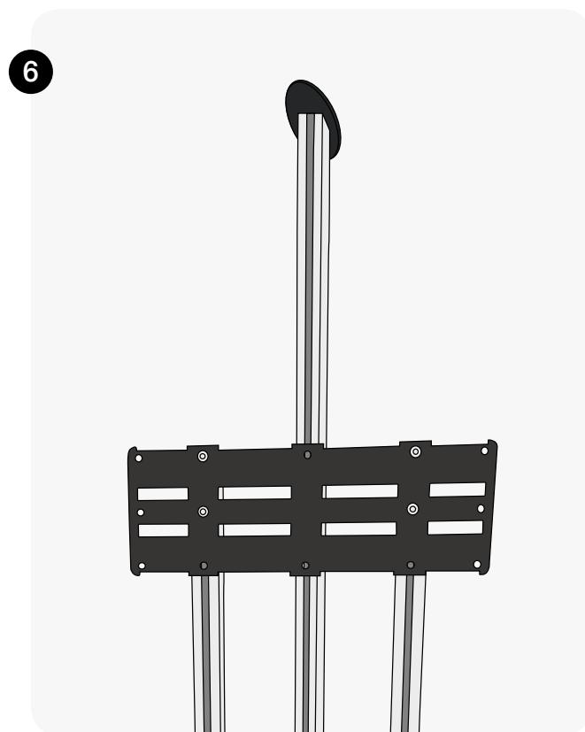
Continue to build the TWIST stand; making sure that the TWIST upright sits behind the AV crossbeam.
