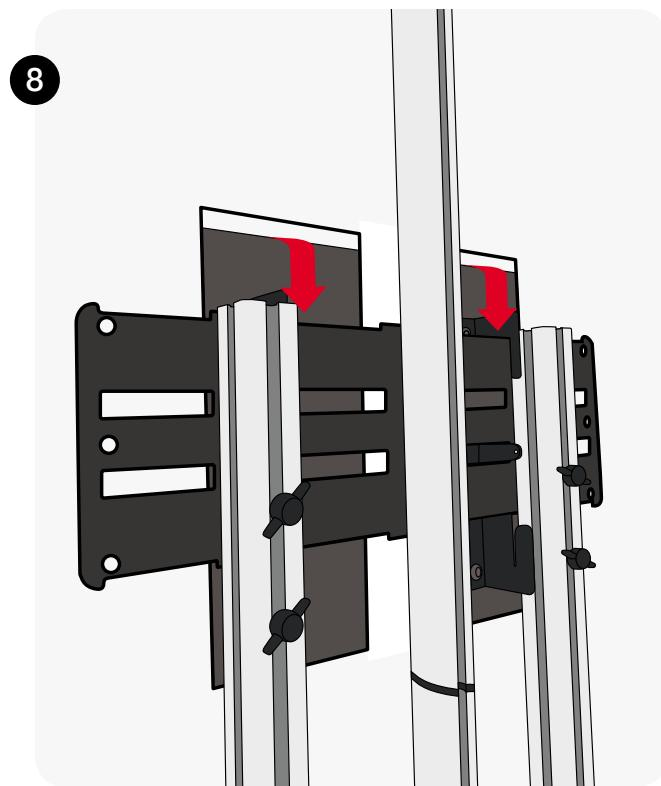
Once you have attached the brackets provided to the TV/Monitor screen, manoeuvre the screen into position so that the two brackets sit on top of the crossbeam. Once the screen is in position, further alterations can be made for cables if required. Then hook the graphic to the base.
