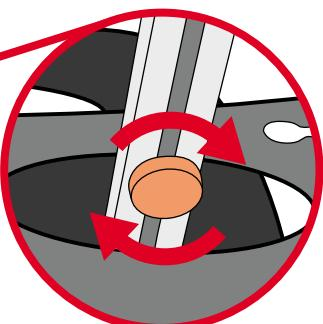
**⚠️ WARNING:** Please ensure orange screws are loosened fully before placing on the base, to prevent the screws resting on top of the locating uprights.
