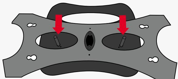
Place a TWIST base over the AV base locating uprights and manoeuvre the TWIST base socket into position.
