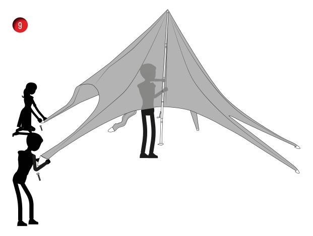
At this stage you can attach the remaining two horseshoe sections of the canopy to the last two ground stakes.
