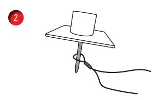
Slide the looped section of the wire setting rope underneath the central stake of the base pole support and temporarily secure it into the ground
