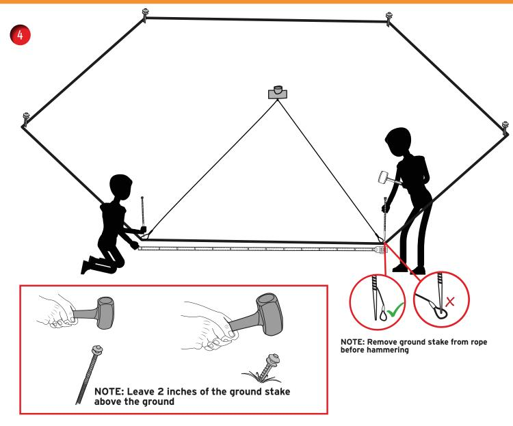
Use a mallet to secure one of the ultra-strong ground stakes into the turf where your two points are marked out, taking care to leave two inches of the stake visible above the ground. Make sure the wire setting rope is loose and is not trapped under or attached to the ground stakes. Repeat steps three and four until you have six points.
