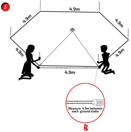
Extend the wire setting rope to full length and separate the two sections of the rope. Use the first section of rope to mark out your first point and take the second section of the wire setting rope and measure 4.9m across from your first point to find the second point of the tent.
