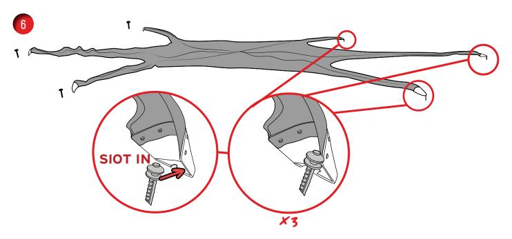
Lay out the canopy of the tent and slot three of the metal horseshoe ends of the graphic around the ground stakes, ensuring the centre of the graphic is draped over the central base support and three of the graphic legs are still free.
