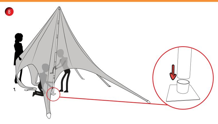
Begin to move the pole into a vertical position until it is straight and the bottom of the pole (part one) can be firmly slotted into the central pole support base.
