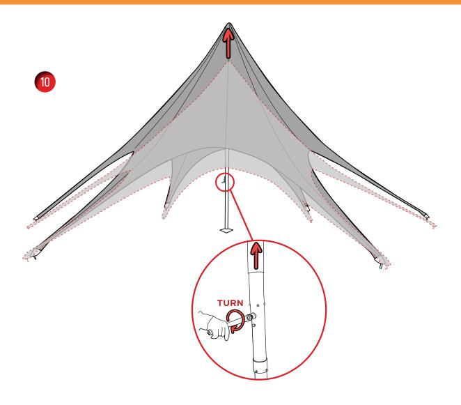
To tension the graphic, turn the crank on the central pole support and, once complete, remove the crank handle.
