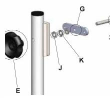
Fix the board plates (G) onto the base legs using a washer (J), spring washer (K), washer (J), and fasten with the M8 bolt (I). Then screw the hand wheel (E) in place. Tighten using the supplied spanner. Repeat for the opposite side.
