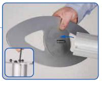
Attach base to male post using M10 bolt and allen key. Ensure clear washer is between base & post. Repeat step for 2nd post.
