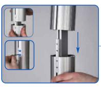
Align and slide female post over male post, tighten both grub screws using a 2mm allen key. Repeat step for 2nd post.
