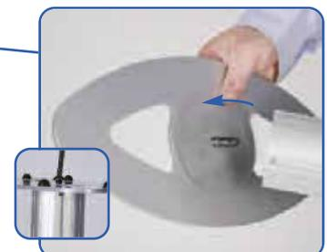
Attach base to male post using M10 bolt and allen key. Ensure clear washer is between base & post. Repeat step for 2nd post.
