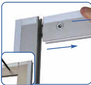
Attach horizontal beams to the vertical frame sides. Tighten locks using a 5mm allen key. If using rigid infill graphics, slide these in to position before tightening beams.
