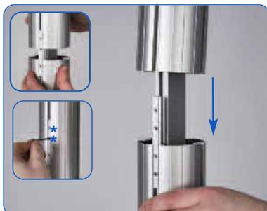
Align and slide female post over male post, tighten both grub screws using a 2mm allen key.
