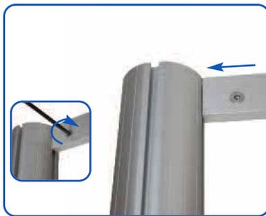
Attach horizontal beams to the vertical frame side. Tighten locks using a 5mm allen key. If using rigid infill graphics, slide these in to position before tightening beams.
