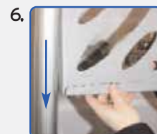
4. Attach leaflet holder to the post. Slide flat bar of holder into the channel of linear post. Ensure thumb fastener threads are flush to the flat bar. Position and angle holder to suit, tighten both thumb fasteners to secure the holder to the post.
