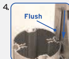
4. Attach leaflet holder to the post. Slide flat bar of holder into the channel of linear post. Ensure thumb fastener threads are flush to the flat bar. Position and angle holder to suit, tighten both thumb fasteners to secure the holder to the post.
