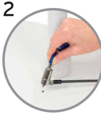
Align and insert end of lock into security slot of LaunchPad base.
