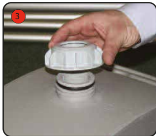
3 Un-fasten the base screws from the base tank.
