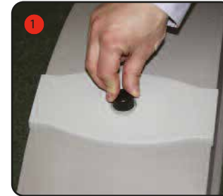
1 Unscrew the 4 base screws from the base tanks and put to one side.
