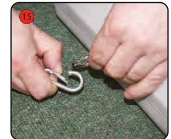
15 Attach the base springs to each base tank ring.
