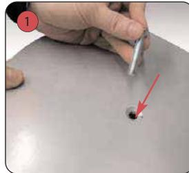
1 Place M8 bolt through the countersunk side of the base.
