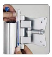
Slide the completed bracket down the post into position and tighten screws to secure.
