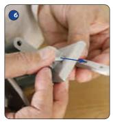
Take the monitor bracket and screw loosely into the linear slider.
