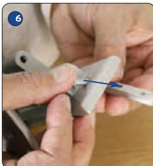
6 Take the monitor bracket and screw loosely into the linear slider.
