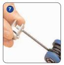
Using a 2.5mm Allen clamping screw in each Poster support.
