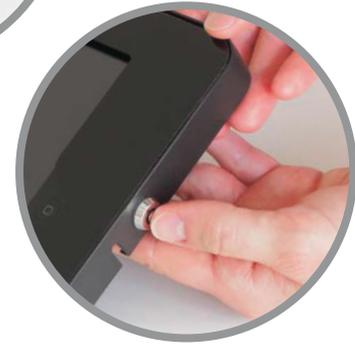
Unlock the iPad enclosure by inserting key into security lock and rotate 'QUARTER TURN ONLY' clockwise or counter-clockwise through 90 degrees which releases the locking pin. Return key back to original position to remove. Lift fascia out of enclosure and place iPad inside, gently pressing all four corners down into mouldings to hold. Replace fascia and depress lock button to secure enclosure.
