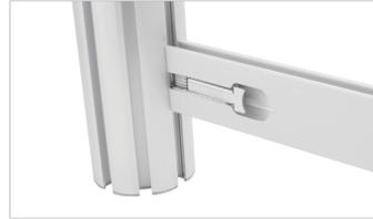
Position 220mm straight T-Loc profiles approx. 150mm from the top and bottom of the 8-way post and at 90° to the cut out in the table top (as pictured bottom left) Insert into 8-way post and secure by shutting clamp lever.
