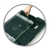
With the elongated holes on the mounting arms lowermost, align arms centrally with 4 off fixing points on rear of screen equidistant from the top. Insert 4 off screws with suitable washers and tighten.
