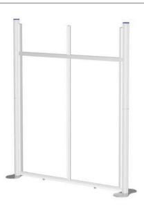
Take final 355mm (V2) profile. Insert T-Loc clamp into channel and line up with joining line of (H) profiles. Close bottom T-Loc lever to secure.
