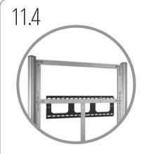
Remove spacer from discarded screw and spacer set, place spacer between connector bar and profile, then insert screw all the way through and tighten to secure.
