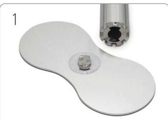
Place base plate on the floor, position lower post centrally over male fitting of base plate (A), and rotate until assembly drops into position, continue rotating clockwise through 90° to secure (B).
