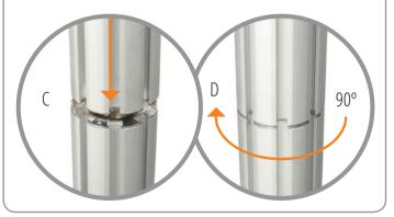
Repeat for remaining base and posts to complete assembly of uprights.
