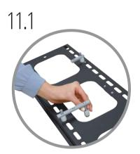
Remove one screw + spacer set from 100mm connector bar on LED/LCD mounting bracket, put aside then loosen other 3 screws slightly.
