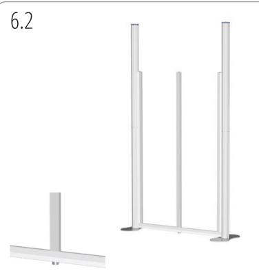
Insert T-Loc clamps into channel and line up with thumb screw foot. Close bottom T-Loc lever to secure.
