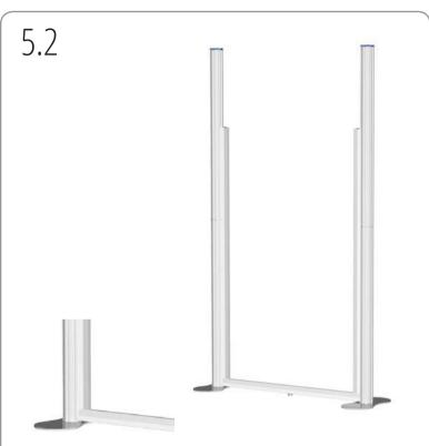
Ensuring the single steel strip of first vertical (V) rail is adjacent to post, slot T-Loc clamp of assembled profile into channel of horizontal (H) at the corner. Close bottom T-Loc lever to secure and repeat for opposite vertical rail.
