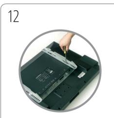
With the elongated holes on the mounting arms lowermost, align arms centrally with 4 off fixing points on rear of screen equidistant from the top. Insert 4 off screws with suitable washers and tighten.
