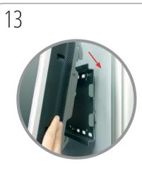
Position screen centrally above bracket and lower until top of both mounting arms hook over mount.
