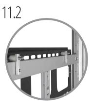
Carefully hook smaller 50mm connector bars over horizontals (H) ensuring they are flush against the profile and straight. The bracket should be central between the posts.
