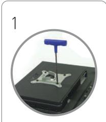
Align VESA mount to rear of monitor, insert 4 off fixing screws and tighten. Arrow on the back of the mount should point towards the top of the monitor.
