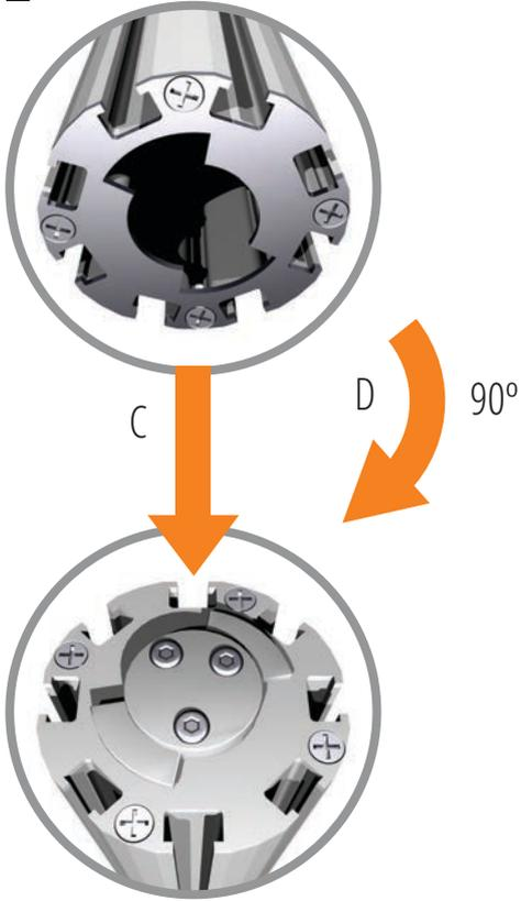
Affix posts (with two brackets) to lower posts by positioning female end centrally over male fitting (C), and rotate until assembly drops into position, continue rotating clockwise through 90° to secure (D). Ensure that all shelf brackets are aligned on one side of the posts (as shown right).
