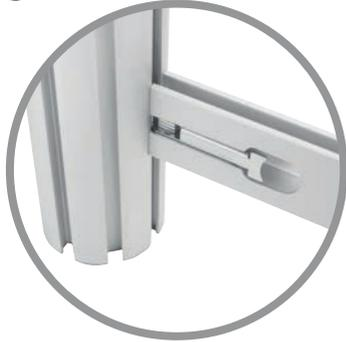
Position post assemblies facing one another with aligned shelf brackets inwards. Connect post assemblies by attaching one of the straight 616mm profiles to the bottom, parallel to the shelf brackets. Slot clamps of profile into post channels and close T-Loc lever to secure.
