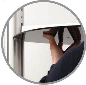
Ensuring the black acrylic is lowermost, slide and raise second assembly into the same post channels as the previous enclosure until the T-Loc clamps come into contact with the bottom of the pre-installed locator bars of the upper posts. Close T-Loc levers to secure in position.
