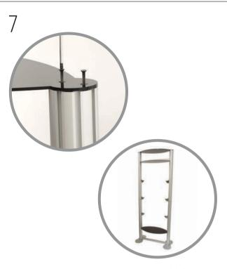
Position top cover onto Centro posts, align countersunk holes with threads within post extrusion, insert 4 off countersunk machine screws and tighten to secure.
