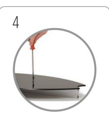
Pre-assemble the two black acrylic shelves to 616mm profiles by aligning the predrilled holes, inserting 4 off countersunk self-tapping screws, and tightening with cross-head screwdriver supplied to secure.
