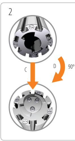
Affix posts (with two brackets) to lower posts by positioning female end centrally over male fitting (C), and rotate until assembly drops into position, continue rotating clockwise through 90° to secure (D). Ensure that all shelf brackets are aligned on one side of the posts (as shown right).
