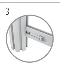
Position post assemblies facing one another with aligned shelf brackets inwards. Connect post assemblies by attaching one of the straight 616mm profiles to the bottom, parallel to the shelf brackets. Slot clamps of profile into post channels and close T-Loc lever to secure.
