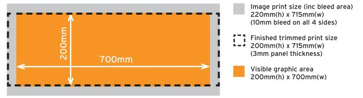
Infill Panels (optional) - Front = 4 panels, Rear = 4 panels - average gap between panels is 15mm
