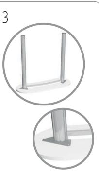
With the steel fixing strip of curved profile adjacent to counter top, slide first curved profile between posts, in channels aligned to cut out of triangular fixing plates.
