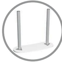
With the labelled '1' end of the post towards the counter top, position female fitting of post centrally over male fitting of triangular fixing plate. Rotate until post drops into position, continue rotating post clockwise through 90° to secure. Repeat for second post.
