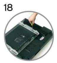
With the elongated holes on the mounting arms uppermost, align arms centrally with 4 off fixing points on rear of screen equidistant from the top. Insert 4 off screws with suitable washers and tighten.
