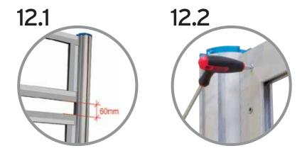
Affix the top section framework into the same channel as the bottom section ensuring graphic fixing strips are all on the same side of the system. Leave a gap of 60mm in between bottom and top framework assemblies and tighten all grub screws in horizontals (H and H1) to secure to post.
