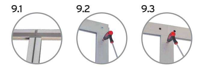
Slot final top horizontal 1500mm rail assembly (H1) to the 220mm verticals, ensuring that the graphic fixing strip is at the top. Tighten grub screws on verticals to secure framework. This completes the top section of the framework.
