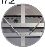
Align other 2 off 260mm connector bars, located behind horizontal rails, and screw into threaded holes. Ensure bottom screws rest on lower horizontal rail, mount is in centre of aperture, and tighten all 4 screws to secure assembly.
