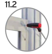
Slot open end of framework into other assembled post, at 90° to the base plate. Ensure bottom section is equidistant from the floor at both ends and the adjustable foot rests on the floor. Tighten remaining grub screws in horizontals (H2 and H) to secure bottom section framework to both post assemblies.
