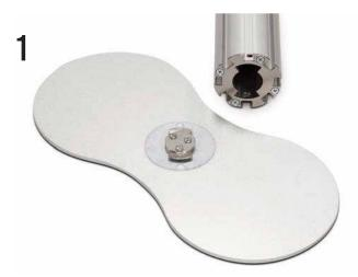
Place base plate on the floor, position lower post centrally over male fitting of base plate (A), and rotate until assembly drops into position, continue rotating clockwise through 90° to secure (B).
