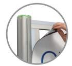
Starting from the top left-hand side of the system, unroll the first graphic panel and align the magnetic tape with the steel fixing strips of the framework. Work across the frame, taking care not to crease the graphic panel. Repeat for remaining graphic panels to complete assembly.
