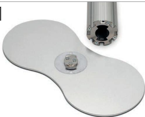
Place base plates on the floor, position lower posts centrally over male fitting of base plate (A), and rotate until assembly drops into position, continue rotating clockwise through  $90^\circ$  to secure (B).
