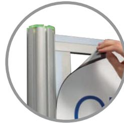
Starting from the top left-hand side of the system, unroll the first graphic panel and align the magnetic tape with the steel fixing strips of the framework. Work across the frame, taking care not to create the graphic panel. Repeat for remaining graphic panels to complete assembly.
