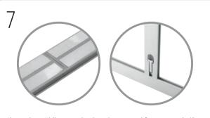
Clamp the middle vertical rails with twin steel fixing strips, halfway across the joins of 750mm bottom horizontal profiles.
