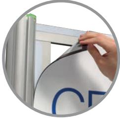
Starting from the top left-hand side of the system, unroll the first graphic panel and align the magnetic tape with the steel fixing strips of the framework. Work across the frame, taking care not to crease the graphic panel. Repeat for remaining graphic panels to complete assembly of the display.
