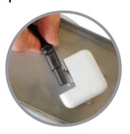
Plug one figure 8 head into a USB Power Adapter (supplied with Apple iPad) and position into retaining pins. Repeat for remaining power leads and adapters.
