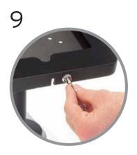
Unlock each iPad enclosure by inserting key into security lock and rotate 'QUARTER TURN ONLY' clockwise or counter-clockwise through 90 degrees, which releases the locking pin. Return key back to original position to remove.
