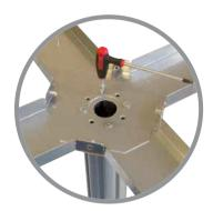
Insert and tighten 4 off base plate screws to secure.
