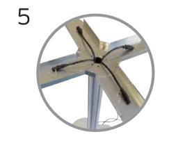
Feed figure 8 heads of power leads through central hole of bottom support plate and carefully place plate onto post. Align 4 holes to threads inside post at desired display angle.
