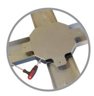
Carefully position and lower octagonal centre cover onto bottom support plate. Align two side holes of cover to any thread fixings of bottom support plate. Insert and tighten two hex socket screws to secure octagonal centre cover.
