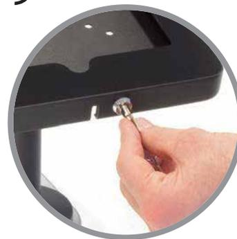
Unlock each iPad enclosure by inserting key into security lock and rotate 'QUARTER TURN ONLY' clockwise or counter-clockwise through 90 degrees, which releases the locking pin. Return key back to original position to remove.
