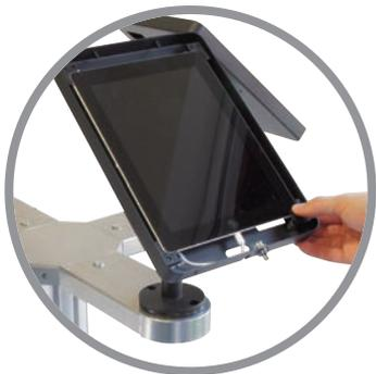
Plug charge/sync cable into one iPad and place inside enclosure, gently press all four corners of iPad down into mouldings to hold. Repeat for remaining iPads.
