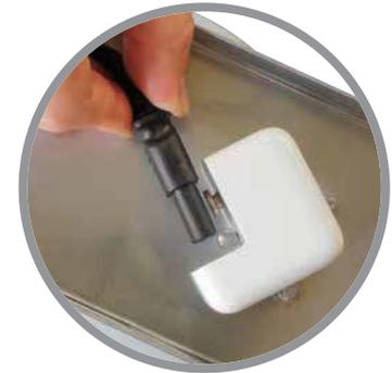
Plug one figure 8 head into a USB Power Adapter (supplied with Apple iPad) and position into retaining pins. Repeat for remaining power leads and adapters.
