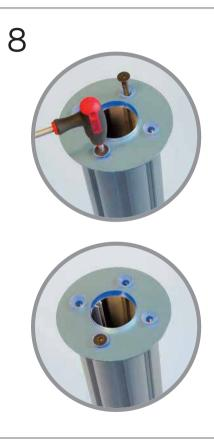
Insert 2 diametrically opposite screws to ensure holes are aligned. Fully tighten 1 screw using hex key provided and once secure, remove opposite screw.
