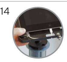
Plug charge/sync cable into iPad and place inside enclosure, gently press all four corners of iPad down into mouldings to hold.
