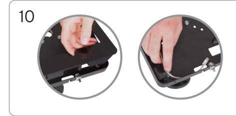
Lift fascia out of enclosure. Insert cable (supplied with Apple iPad) allowing 10cm to remain "free" at charge/sync connector end by gently pressing into retaining moulding.
