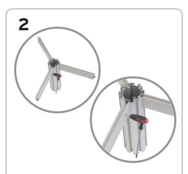
Take 265mm post and slot clamp of three 220mm profiles into desired channels for display. Ensure bottom of profiles are flush with bottom of post and tighten grub screws to secure in position.
