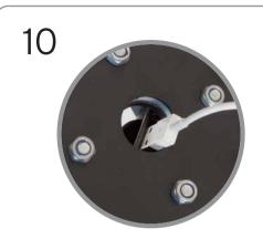
Feed USB end of charge/sync cables through middle of enclosures, below pin, so they protrude from bottom of support columns.
