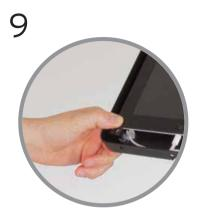
Plug charge/sync cable into iPad and place inside enclosure, gently press all four corners of iPad down into mouldings to hold.
