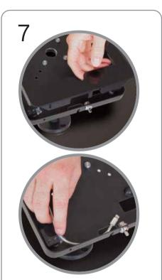
Lift fascia out of enclosure. Gently press cable (supplied with Apple iPad) into retaining moulding, allowing 10cm to remain "free" at charge/sync connector end.
