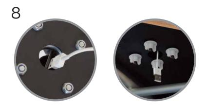
Feed USB end of charge/sync cable through middle of enclosure, below pin, so it protrudes from underside of counter/table top.
