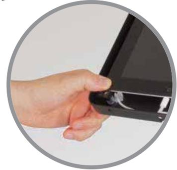
Plug charge/sync cable into iPad and place inside enclosure, gently press all four corners of iPad down into mouldings to hold.
